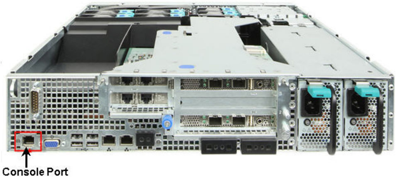
FIGURE 2 SZ300 Location of console port
